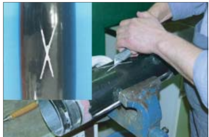
Fig. 7: DENSOLID FK2: V-cut lift-off test after water immersion - no loss of adhesion, rupture occurs within coating
